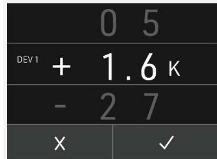
10. In the calibration settings, set the compensation correction value for **CAL1** to +1.6 K (measured actual value minus setpoint = correction value).
